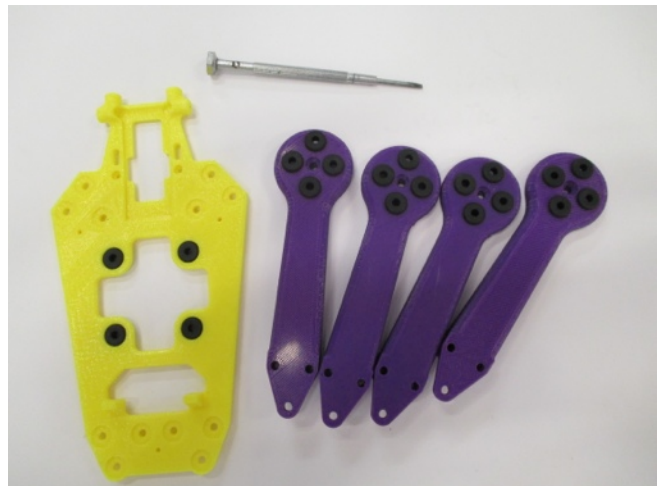
Grommets installed. The jeweler's screwdriver shown works well for seating the grommets,
